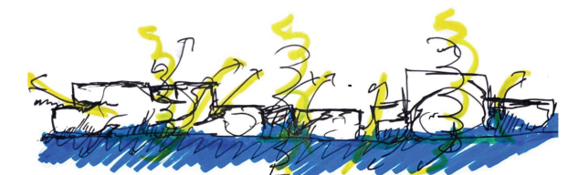
Building in Section A-A air enters air exits air goes through cross and makes a convection cell in cross space between
